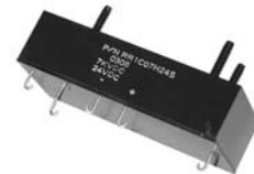
RR1C07H24S SPNO 7kV PK TEST HOOK, SOLDER TERMINALS 24V DC ACTUATOR STUD MOUNTING
